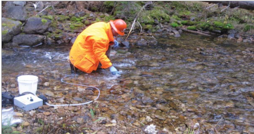
Stream water is pumped through a filter which is then analyzed for DNA from the species of interest.
